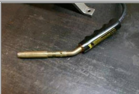
I tried several different torch outfits and settled on using a Bernz O Matic model # JTH7, it seems to produce the best heat and has the added flexibility of the separate torch wand. This picture is of the torch wand removed from the forge. I got the torch outfit at Home Depot for less than \$30.00.
